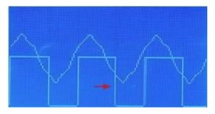
If the falling edge is to the left of the bottom peak, move the sensor to the right.
