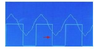
If the falling edge is to the left of the bottom peak, move the sensor to the right.
