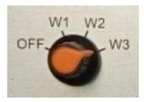
If no signal appears, set the switch to positions W1, W2, or W3
