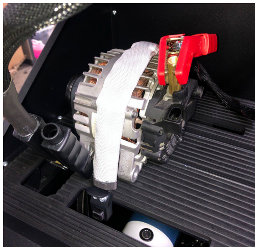
Figure 16. Connection of Power Wires to the Alternator
