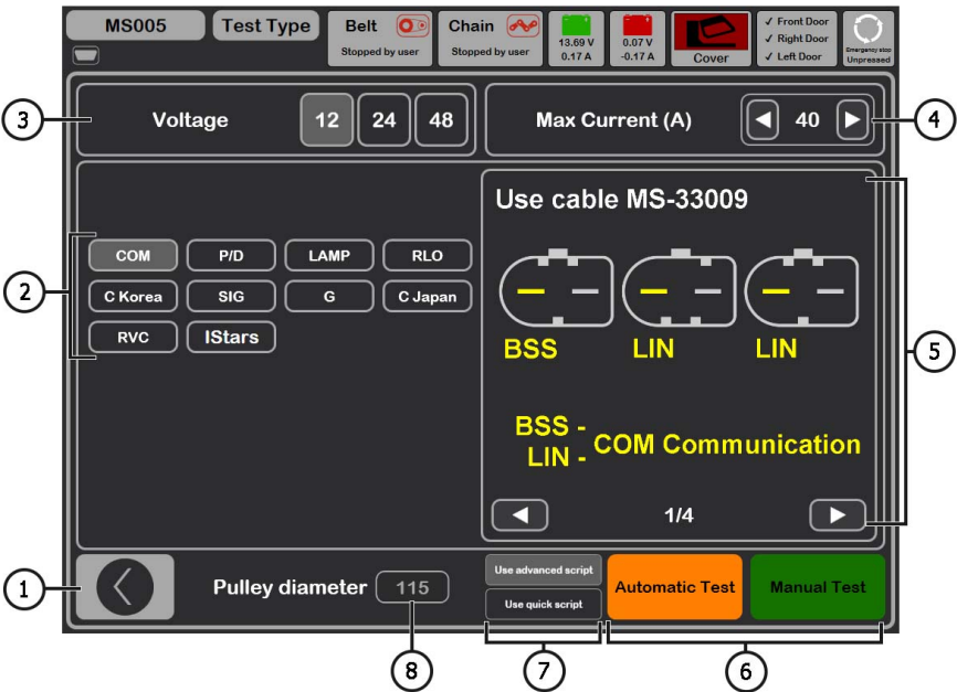
Figure 22. Menu for Selecting the Diagnosed Alternator Type
