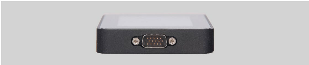
Figure 2. Terminal for connection of diagnostic cables
